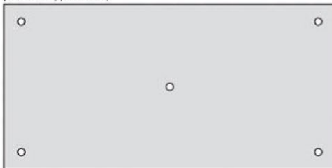
5 insulation fastener pattern (suspended ceiling/no external wind pressure applications)
