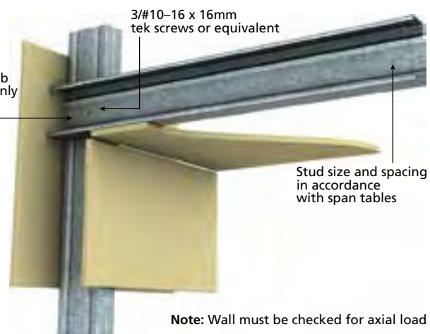
MECHANICAL JOINT TYPE 3
